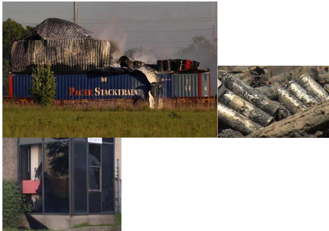
Figure 4 Explosion of container filled with consumer Li-Ion batteries during rail transport
