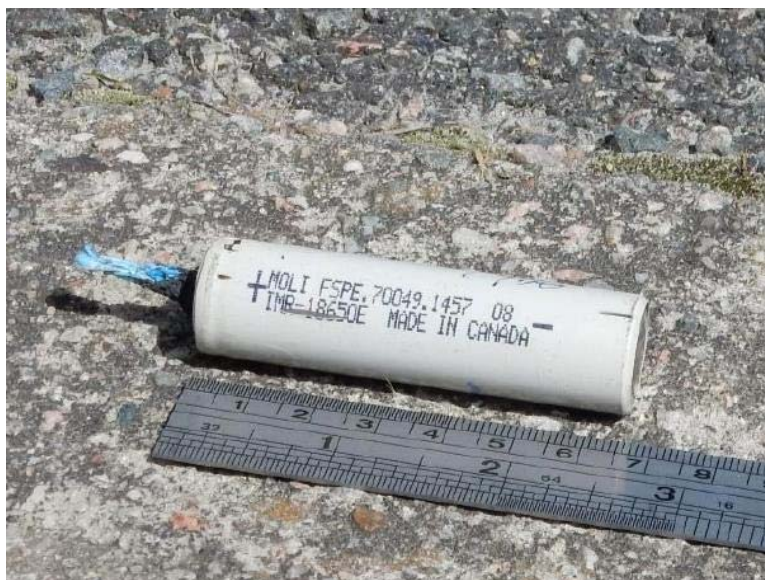
Figure 19 Picture of an 18650 Li-Ion battery after thermal runaway
